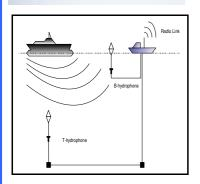
The PUAMS-SS03 system is modular, manufactured from COTS components and consists of the local measuring subsystem, the remote data processing subsystem and various optional accessories according to the specific customers requirements.
